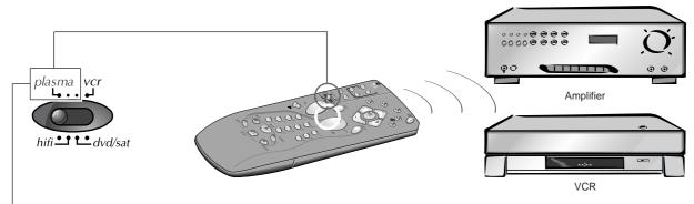
When the switch is on the plasma position, some of the keys control the devices indicated on this page. For other devices (Amplifier, DVD, Satellite and VCR), refer to pages 31.
